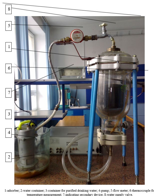
Figure 4. Experimental installation for adsorption purification
