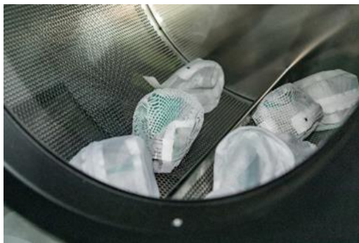
Figure 3. Interior of the VDHO3 system with FFP2 masks and their cover
