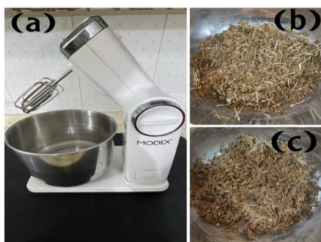
Figure 4. (a) An electric mixer; (b) Soil mixed with SCF; (c) Soil mixed with PPF
