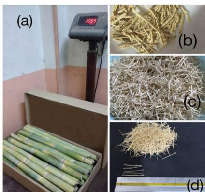
Figure 2. Created fibers: (a) From the supplier; (b) Cutting the hard outer rind of the sugarcane; (c) After the process by washing and drying; (d) After cutting to a specific length
