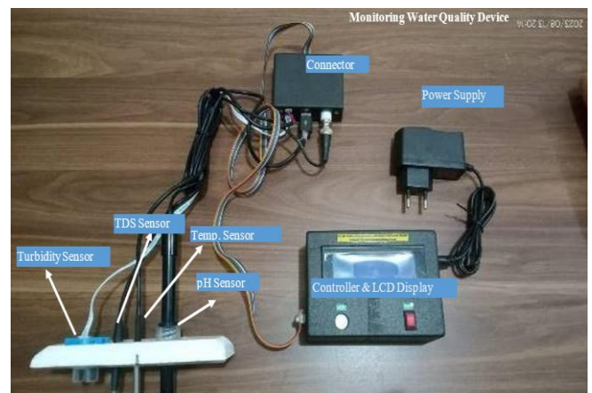
Figure 6. Prototype of pond water quality monitoring hardware
