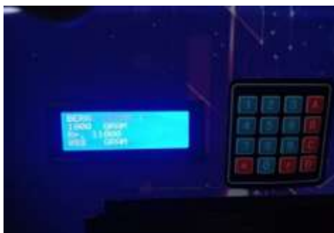
Figure 7. Keypad and LCD I2C function testing
