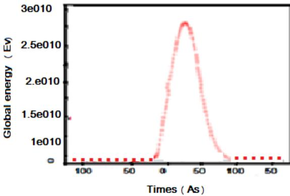
Figure 3. The time evolution of global energy Xe ( $3.10^6$ ),  $I=10^{21}$  W.cm $^{-2}$ ,  $\lambda=390$  nm and  $\tau=150$
