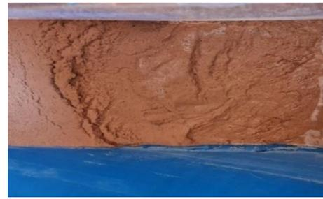
Figure 16. Upstream slope erosion of anisotropy model dam after sudden draw down
