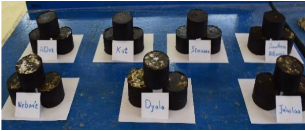
Figure 4. Prepared samples by Marshall compaction
