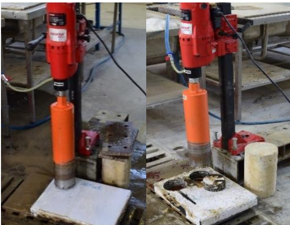
Figure 6. Pre-and post-coring samples in lab
