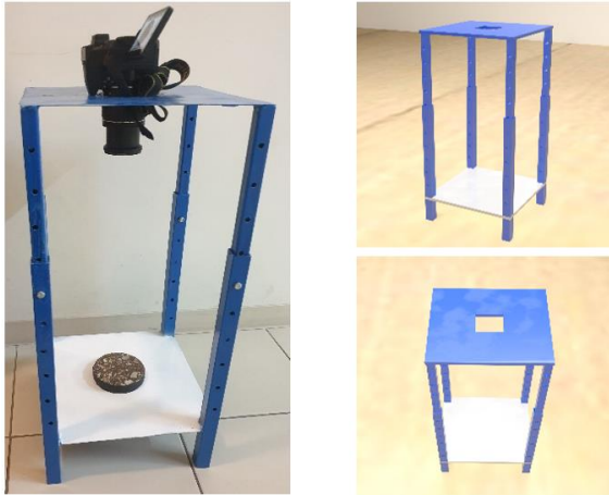
Figure 9. Manufactured steel frame (Images calibration)
