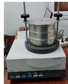
Figure 2. RETSH AS 200 vibratory sieve shaker
