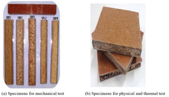
**Figure 6.** Sandwich structured composite specimens
