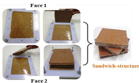
**Figure 5.** Protocol for the preparation of new sandwich-structured composite plates
