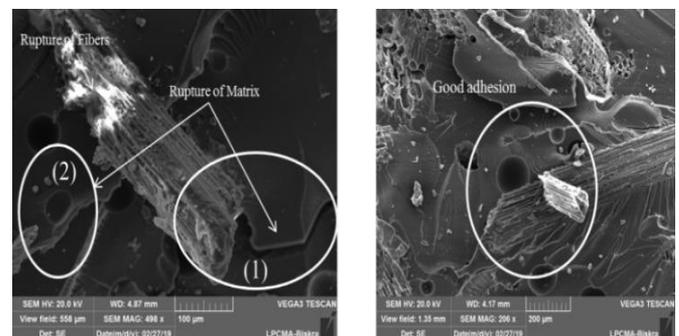
**Figure 14.** SEM micrographs of the skins after the three-point bending test
