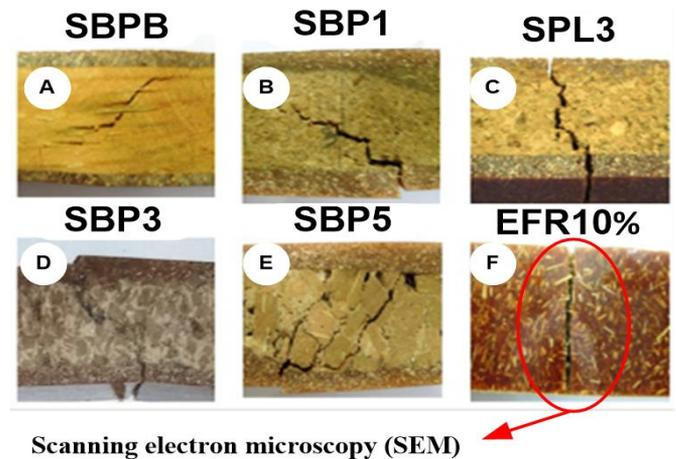
**Figure 13.** Macroscopic observations of the fracture surfaces of the various sandwich structures
