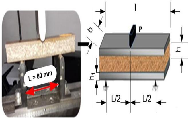
**Figure 7.** Sandwich beam specimens in three-point bending test
