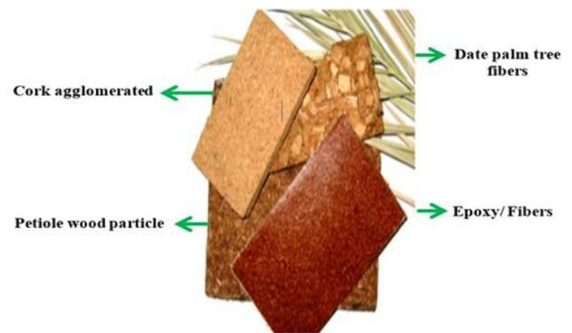
Figure 2. Materials used in novel bio-composites with a sandwich structure
