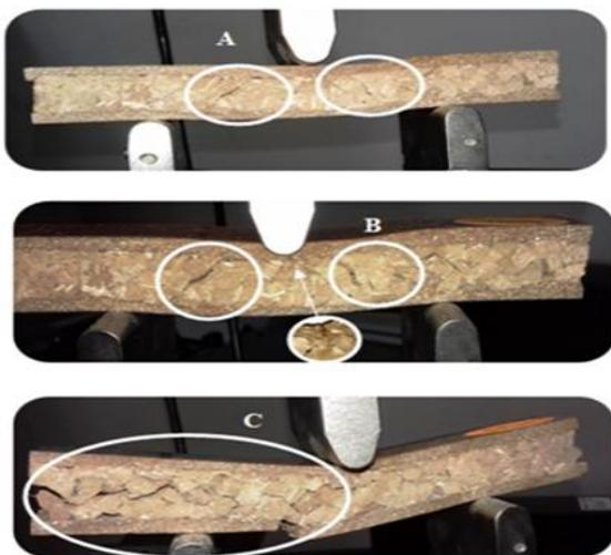
**Figure 12.** Macroscopic observations of the fracture stages of a specimen
