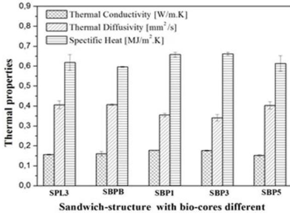
**Figure 9.** Thermal properties of new sandwich-structured composite with different bio-cores
