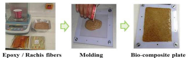
Figure 3. The main preparation steps of (EFR10) are used as the skin of the new sandwich-structured composite
