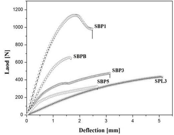
**Figure 10.** Example of load-displacement curves during three-point bending tests on different sandwich-structured composite beams
