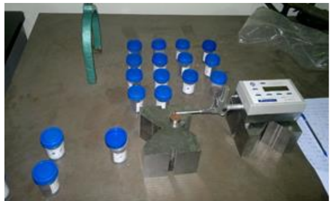
Figure 7. Taylor-Hobson surface roughness tester used in this study
