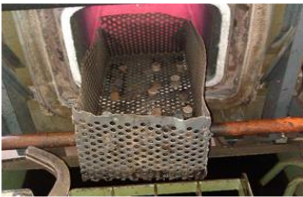
Figure 5. Furnace used in this study for heat treatments
