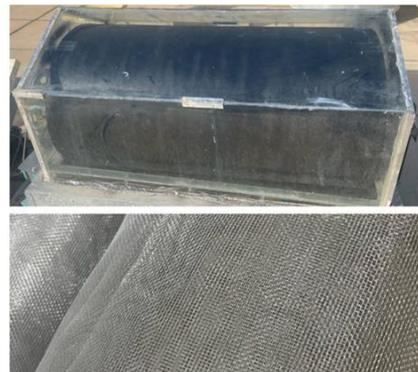
Figure 2. Before and after painting the aluminum mesh with an opaque black for coated the rotating hollow cylinder
