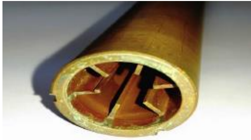
Figure 4. Photographic view of condenser with fins attached internally [31]
