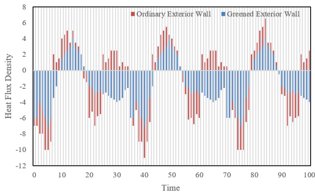
Figure 7. Comparison of instantaneous heat flow transmitted from exterior walls to indoors
