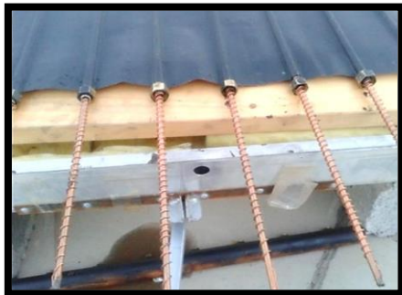
(b) Helical spring inserted inside thermosiphon riser collectors
