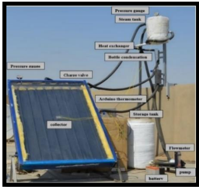
(a) The photo of the indirect solar water heating collector including a thermosiphon
