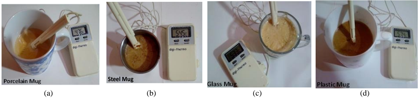
Figure 9. Experimental set up for recording time dependent thermal profile of cooling tea for: (a) porcelain mug, (b) stainless steel mug, (c) glass mug, (d) plastic mug of tea
