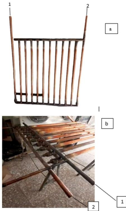
Figure 7. Phytophagic of solar collector models (FPC): (a) SRT 1 . 1 and 2, Inlet or outlet fluid; (b) SRT 2 . 1 and 2, Inlet or outlet fluid
