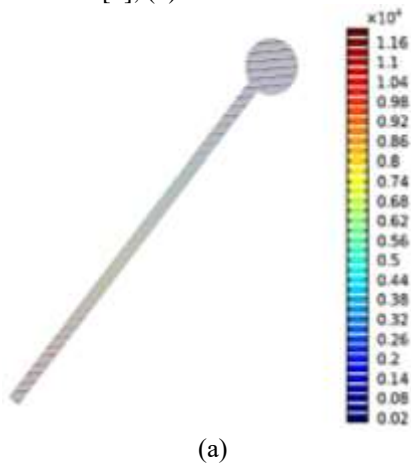
Figure 10. Temperature profile of the ETSC water heater with 26 Lit tank capacity. (a) Gholamabbas et.al work (2020) [8], (b) Present work
