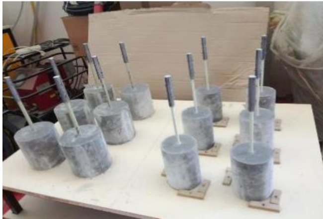
Figure 4. Anchor heads of the GFRP rebars
