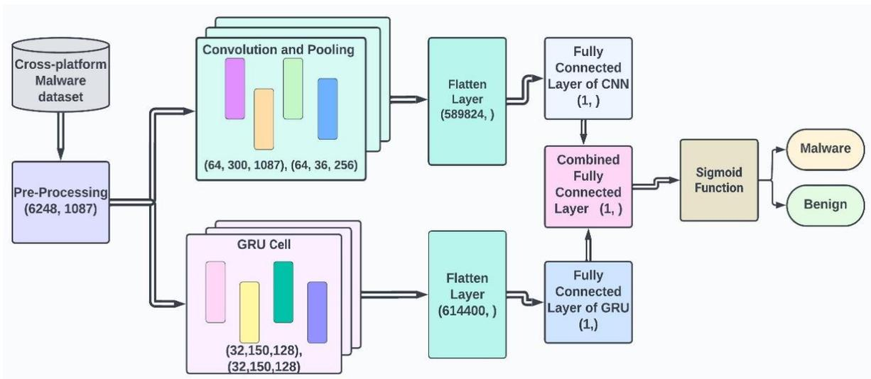
Figure 2. CNN-GRU architecture for cross-platform malware classification
