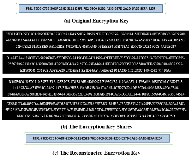
Figure 8. (a) original encryption key, (b) the shares of the secret key after applying the Shamir secret sharing scheme of (3,4) threshold, (c) the reconstructed encryption key
