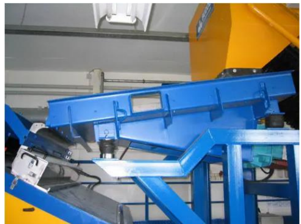
Figure 6. Vibrating conveyor Source: Compiled by the authors
