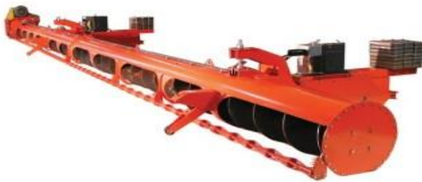
Figure 3. Screw (auger) type conveyor Source: Compiled by the authors
