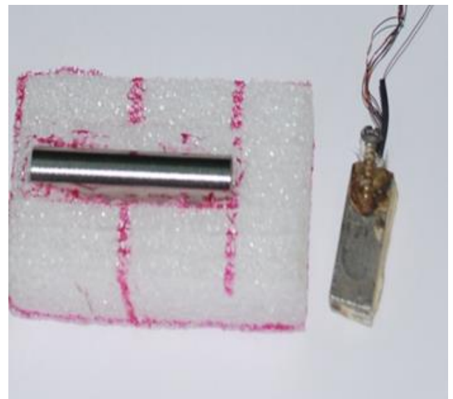
Figure 13. Picture of cylindrical specimen along with PEC sensor
