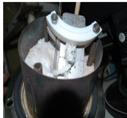
Figure 7. Different perspective view of canned PEC probe with test specimen and sand witted SS shims in crucible
