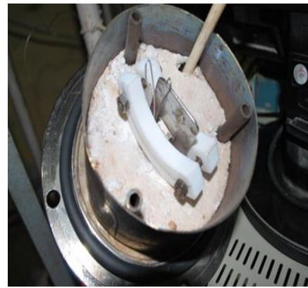
Figure 6. Picture of canned PEC probe with test specimen and sand witted SS shims in crucible
