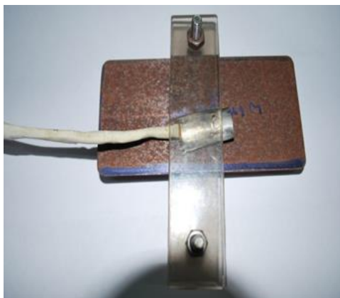
Figure 18. PEC sensor testing on a ferromagnetic test specimen
