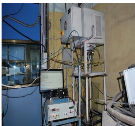
Figure 5. Picture of a different perspective view of high temperature experimental test setup for canned PEC probe testing
