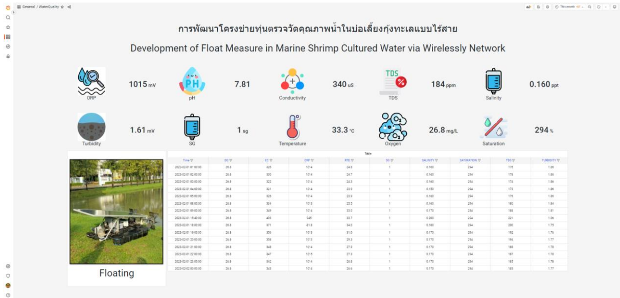
Figure 9. pH, temperature, DO, Conductivity, ORP, Salinity, TDS, and turbidity via the web application
