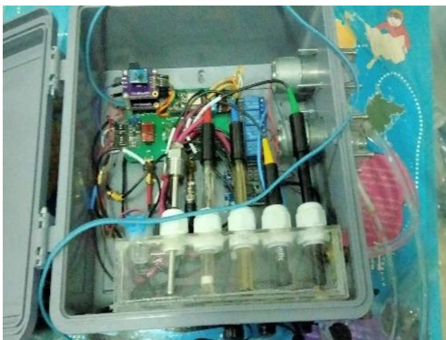
Figure 3. The sensor box used for water quality measurement
