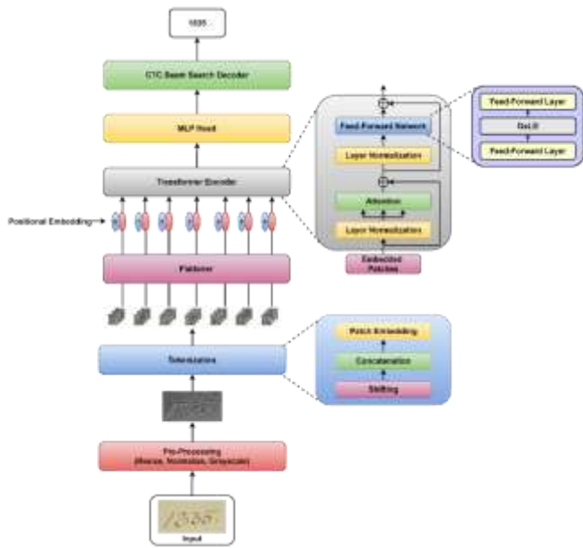
Figure 3. The proposed architecture of Decoded-ViT for HDSR
