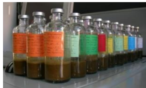
Figure 1. Picture of batch digesters
