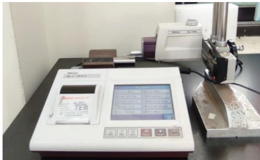
Figure 3. Measuring roughness with the SJ-410
