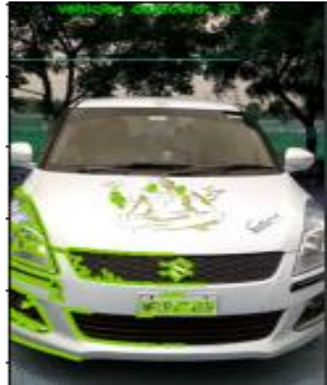
Figure 17. Detected contours in the frontal view of a White Maruti Swift Vehicle
