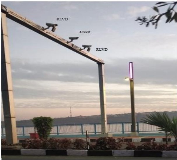
Figure 5. Camera set-up of ITMS at road-side traffic area
