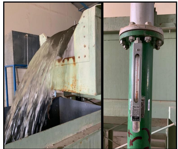
Figure 4. The instrument for measuring the discharge
