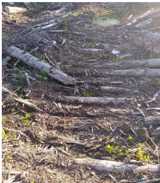
Figure 1. Crushed and indented logging residues on the skidding trail in the cutting strip (Krasnoyarsk Krai) [15]
