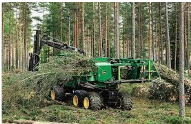
Figure 10. A machine for harvesting and bundling logging residues on a cutting strip
