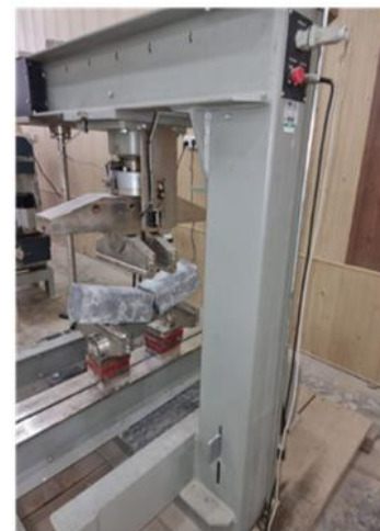
Figure 4. Flexure test equipment
