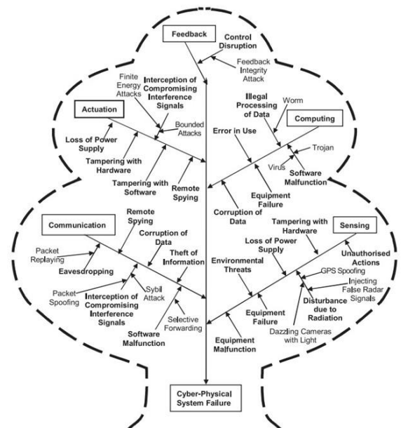
Figure 3. A tree diagram representing attacks and threats on cyber-physical systems (CPS) [29]
