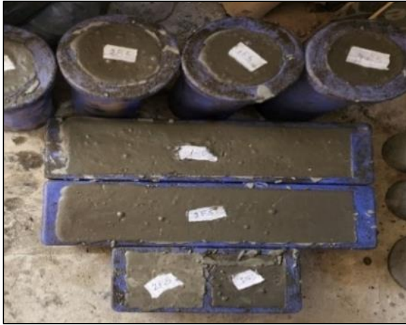
Figure 2. The SIFCON specimens pouring procedures
