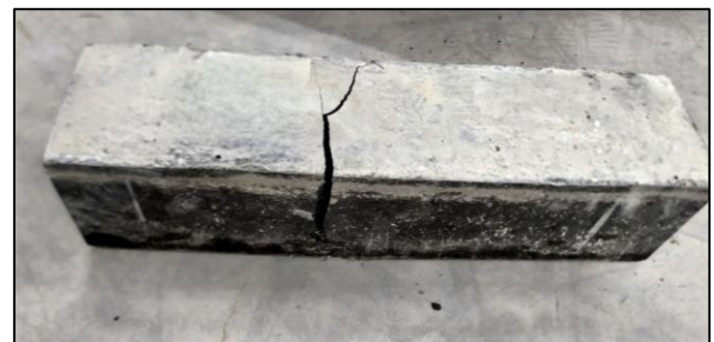
Figure 6. Flexural failure mode of SIFCON samples
