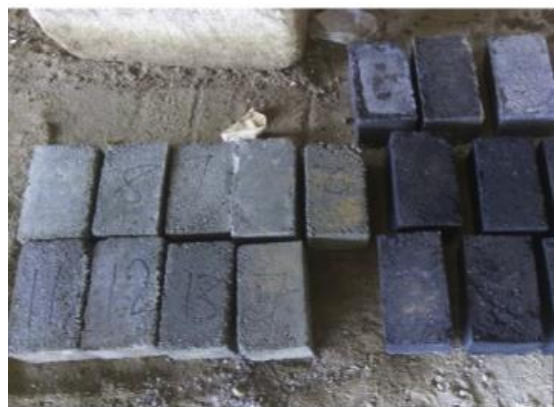
Figure 4. Recycled plastic waste as pavement blocks (Agyeman et al. [8])
