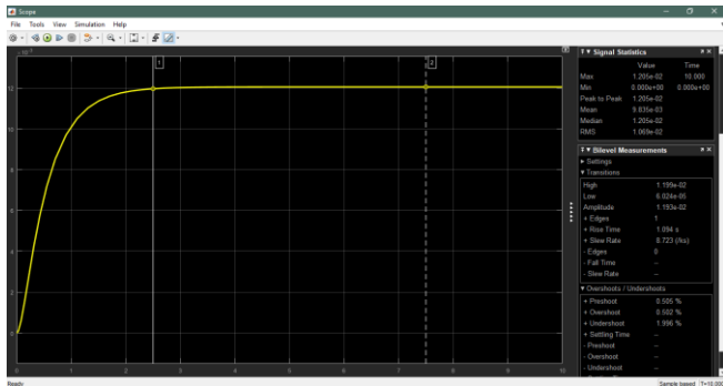
Figure 8. Open loop transient response of DC motors
