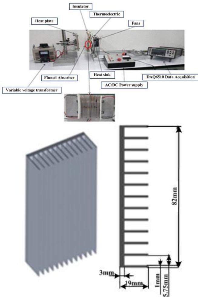
**Figure 1.** The experimental setup (top) [15] and geometry and dimensions of the RVFA (bottom)
