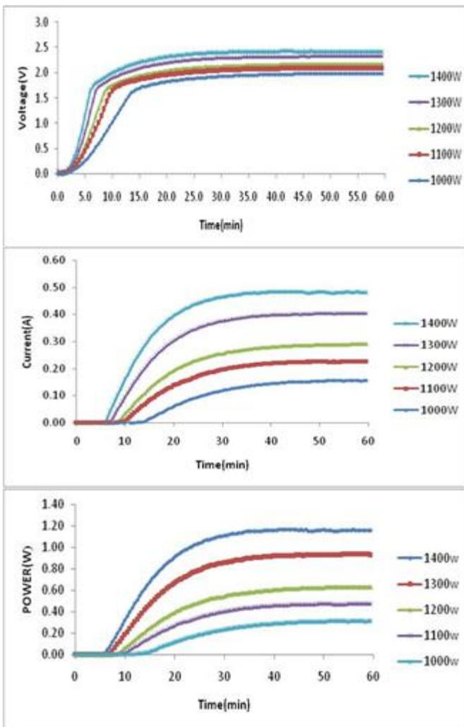
**Figure 3.** Variations of measured electrical parameters versus time for the various power applied at 3 cm air gap
