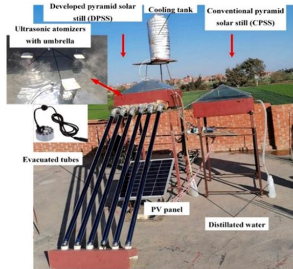
Figure 5. Pyramid solar still with ETC
