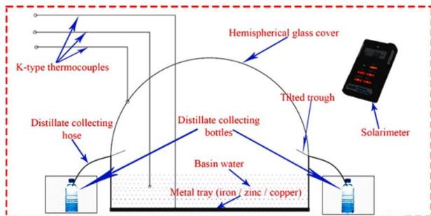
**Figure 3.** A traditional hemispherical solar basin's 2D design [23]
