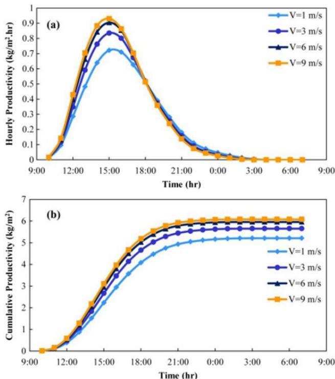
**Figure 6.** Basin solar still output (a) hourly (b) accumulated at various wind speeds [46]
