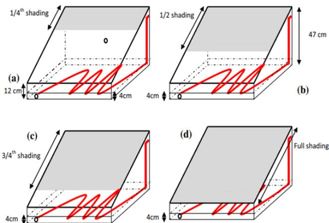
**Figure 9.** The glass cover provides shading and cooling to different proportions of the surface area, including 1/4th, 1/2nd, 3/4th, and the full area [69]
