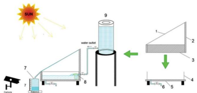
Figure 1. One-slope solar distiller [17]
