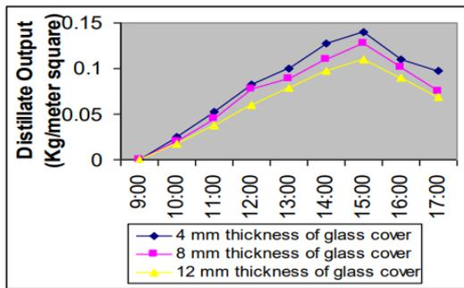
Figure 7. Solar still distillate yield is affected by glass cover thickness [57]
