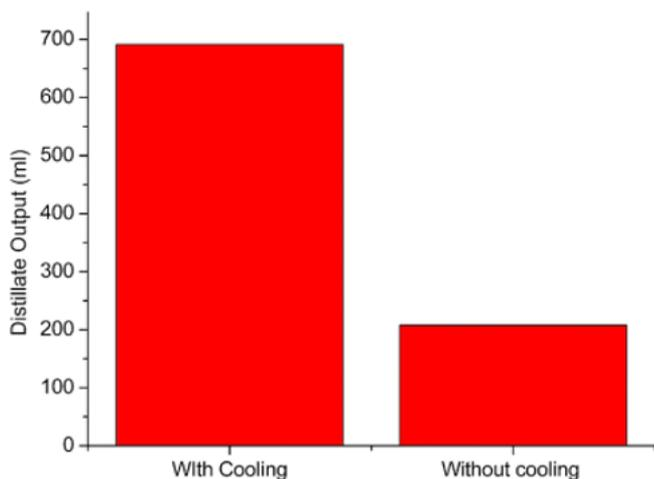
**Figure 8.** Comparison between the production of distillate in a solar still, with and without the utilization of a glass cover to facilitate cooling [69]
