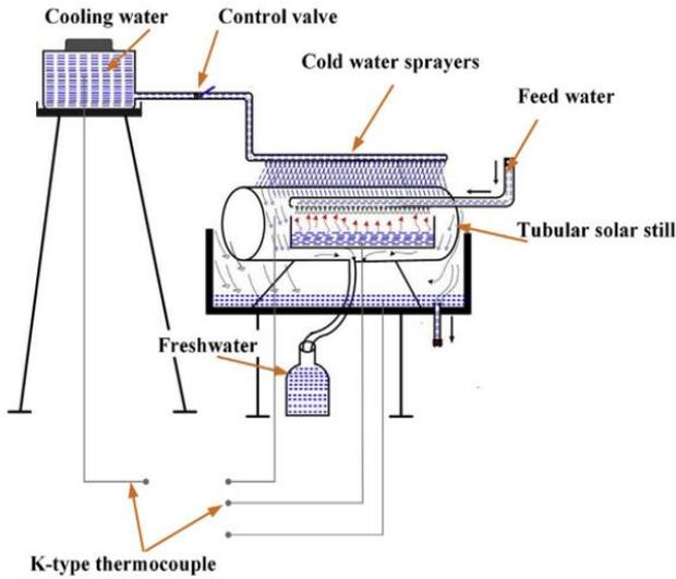
**Figure 2.** Solar still with a tubular design [23]
