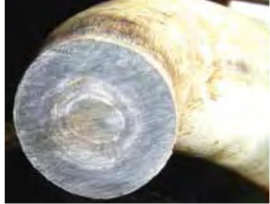
Figure 3. The cross-section of the horn has a concentric structure [41]
