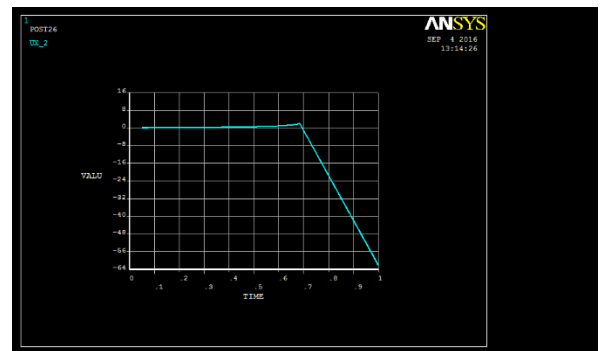
Figure 9. Displacement vs time graph for non linear buckling analysis of al-cu alloy conical shell
