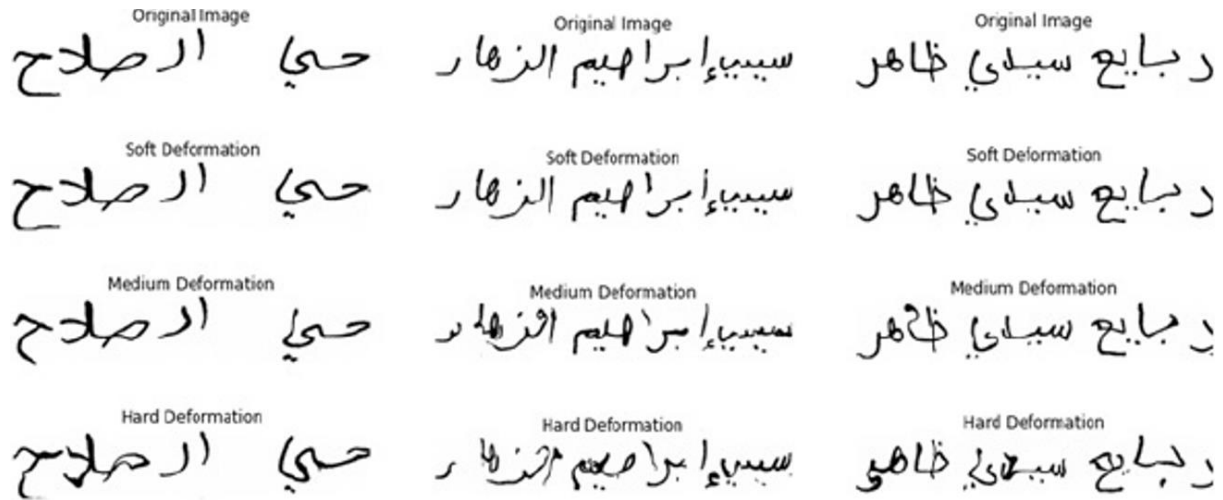
Figure 5. Three examples of augmented images using the MLS augmentation technique with: Soft deformation, medium deformation, and hard deformation
