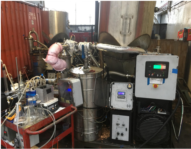
Figure 2. ALL power labs power pallet with on-line tar tester
