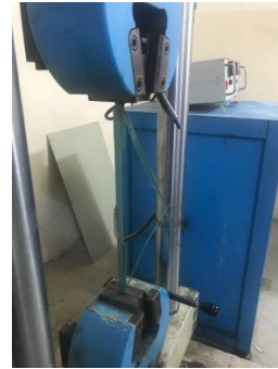
Figure 2. Strapping ties under tensile strength test
