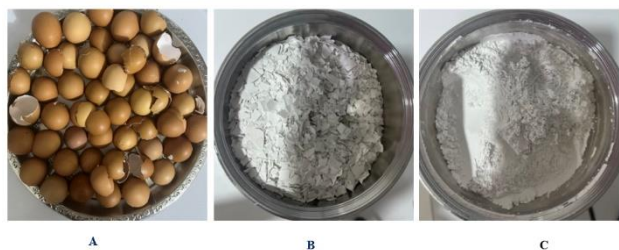
Figure 2. Procedure for making HA powder from eggshells: (A) Egg shells cleaned; (B) Broken and calcinated egg shells; (C) Crushed and milled egg shells
