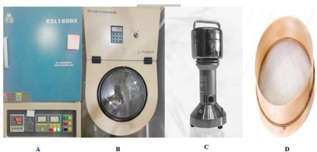
Figure 3. The tool used to make HAP powder from eggshells: (A) furnace, (B) planetary ball, (C) home steel mill, and (D) sieve
