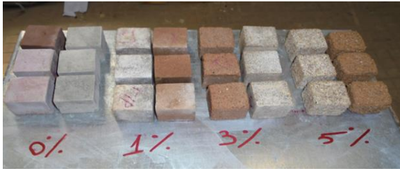
Figure 11. Visual appearance of GM and PM before and after 28 days to exposure to 1%, 3% and 5% sulphuric acid solution
