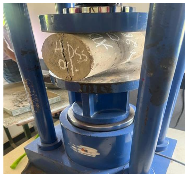
Figure 2. Split tensile strength test
