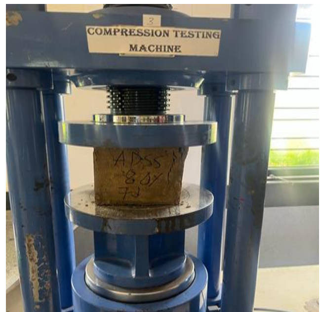
Figure 1. Compressive strength test
