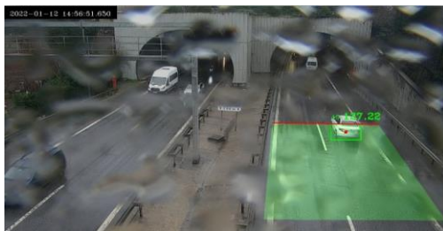
Figure 39. Incorrect vehicle and speed detection under heavy rain (zoomed)
