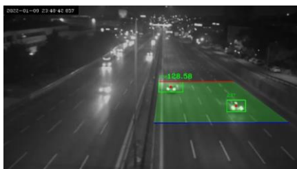
Figure 40. Vehicle detection with low image quality
