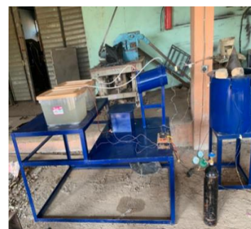
Figure 7. The fabricated batch reactor assembly
