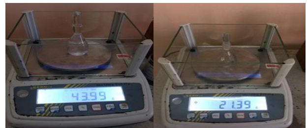
Figure 4. Density measurement of oil
