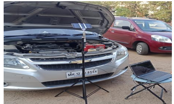
Figure 22. Car engine vibration video recording setup
