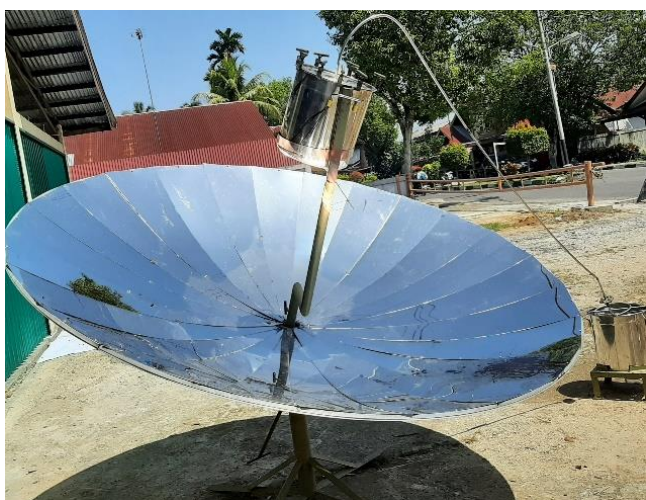
Figure 2. Parabolic solar pyrolysis
